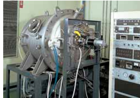
Photo 4.1 Vacuum testing system
