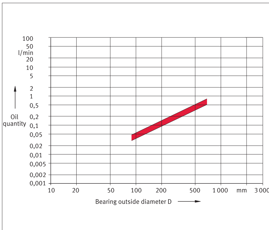
17: Minimum oil flow rate for spherical roller bearings of series 223 in vibratory machinery
